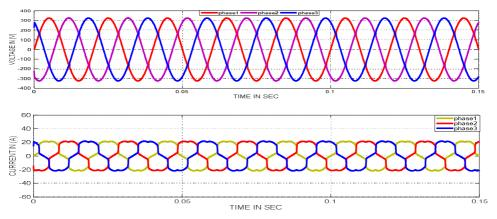
Fig. 9 Voltage and Current Waveform with C-types high pass filter Harmonic Filters.
