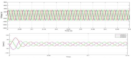
Fig. 13 Voltage and Current Waveform with Active Harmonic Filters.
