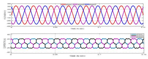
Fig. 7 Voltage and Current Waveform with Single Tuned Harmonic Filters.
