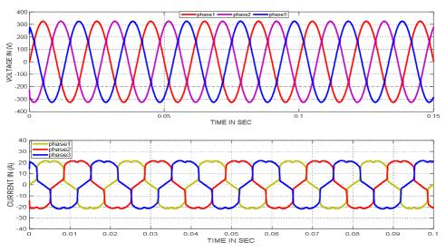
Fig. 5 Voltage and Current Waveform with Double Tuned Harmonic Filters.
